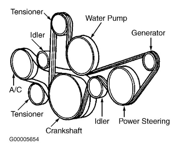
Fig. 1: Serpentine Belt Routing Courtesy of GENERAL MOTORS CORP.
